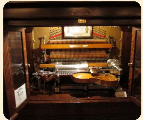
The interior of the Mills Violano with the violin and piano action.
