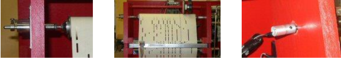
Here a 58n roll is mounted. The right pic shows the 58n chuck installed and locked. The left pic shows how the left idler chuck compensates under spring pressure. The center pic shows the roll centered.
