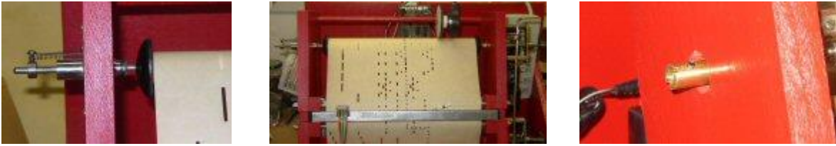
Here a 65n roll is mounted. The right pic shows the 65n chuck installed and locked. The left pic shows how the left idler chuck compensates under spring pressure. The center pic shows the roll centered.
